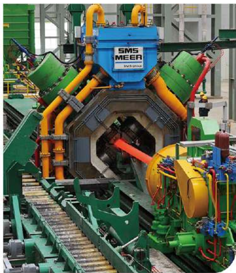
16MN 精锻机 16MN PRECISION FORGING MACHINE
