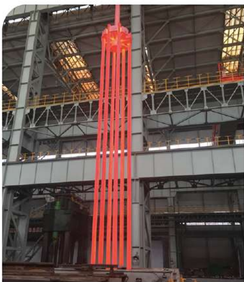
井式调质生产线 WELL ROLLER-TYPE QT LINE FOR FLATS
